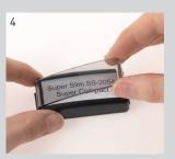
Select right colour of MaxLight Let ink soak in and put index card and cover lens back in place. Wait 45-60 minutes for ink to migrate and test stamp. Repeat steps if necessary.
